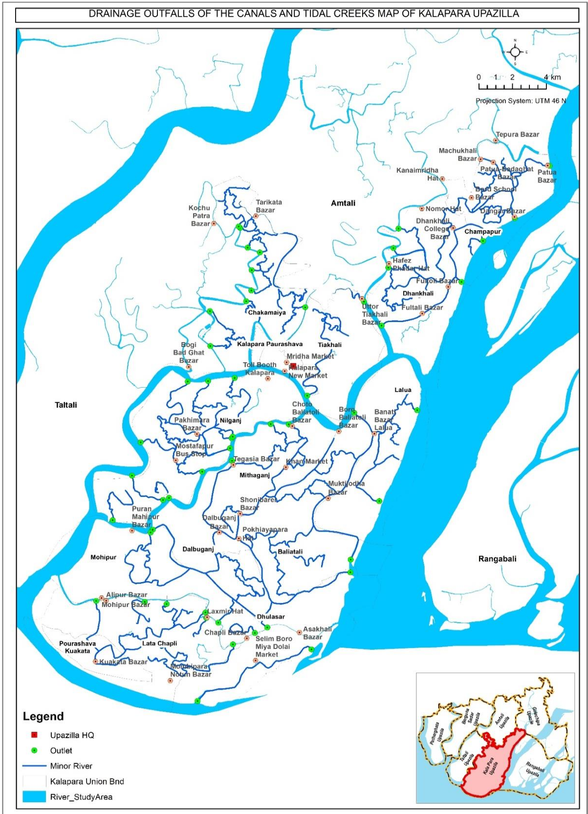
Figure 20: Existing Natural Drainage Network and Outfall
